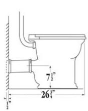
When W.C. pan is set at MINIMUM distance from wall.
