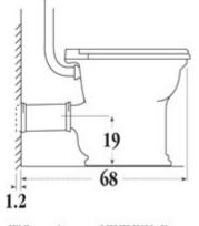
When W.C. pan is set at MINIMUM distance from wall.
