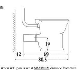
(For when connecting to an existing soil pipe which projects
