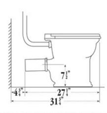
When W.C. pan is set at MAXIMUM distance from wall.
